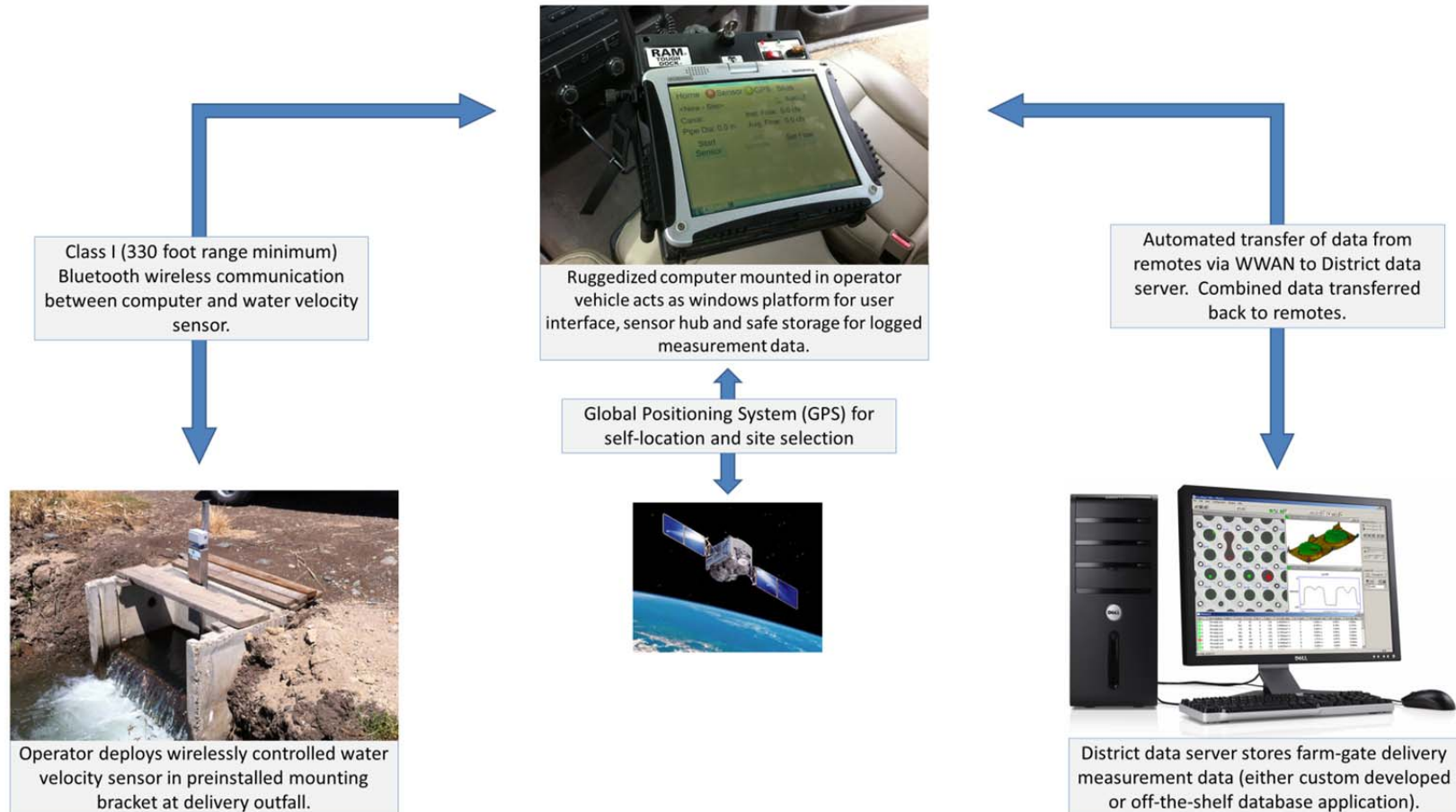
Figure 2. RemoteTracker Principles of Operation Overview
